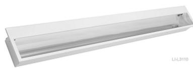
Asymmetrical batten luminaire with laterally inclined light emission for wall lighting, corridor, shop, gallery. Installation in hollow ceilings, for 1x fluorescent lamp 54W. With aluminium reflector, electronic ballast.
